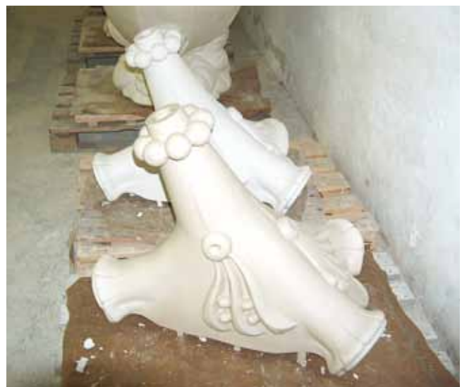
6. Special ridge tiles made of pyrogranite, before glazing
